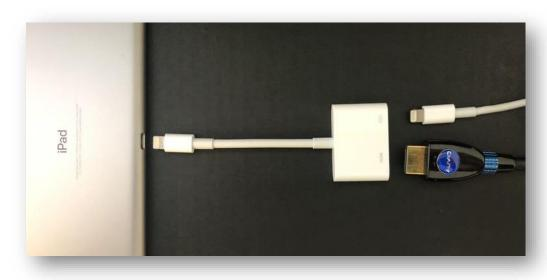
The *advantages* of a wired setup is that the you should see the iPad's screen on the TV or projector almost immediately, and the video stream will be more reliable.
